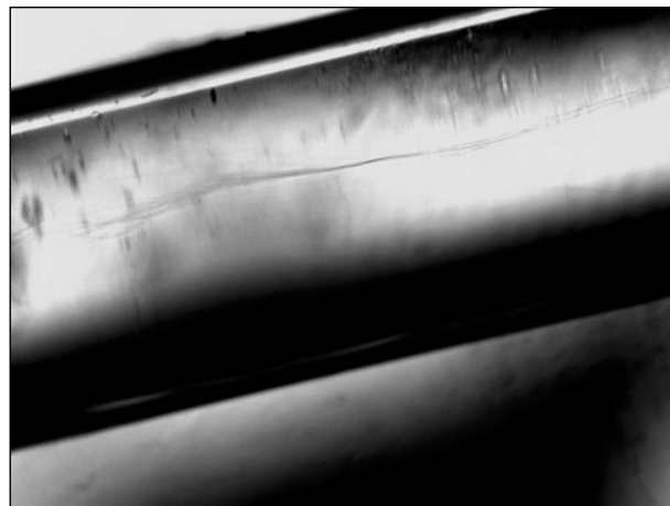
Fig. 3. Discrete set of strings formed in a capillary with a diameter of 300 \mu . \times 200 .
